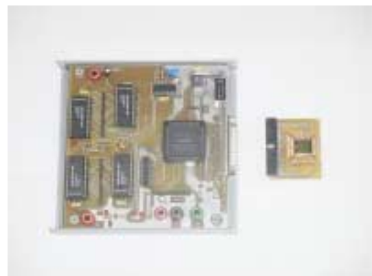
Figure 6: First discrete implementation of proposed electronic system architecture: analog and digital control system circuitry in the left side and connected first 4x4 micro-rockets array in the right side.
