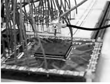
Figure 3. Injecting the transient fault caused by electromagnetic waves from the short-circuit discharge of a capacitor
